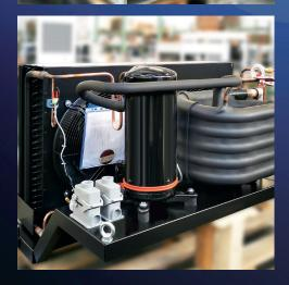
Built-in fluid cutting fluid cooler, without metal frame, nominal cooling capacity 12 kW.
